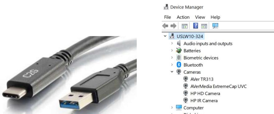
**USB Connection (TR313V2):** Connect the AVer TR313V2 Camera to a USB port on the PC using a Type-B USB cable to Type-A/C USB cable and verify that Windows does see the device in the “Device Manager” window.
